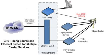
sharing base station equipment and separate TDM circuits need to be accessed per carrier. Without a local source of Stratum 1 timing, these circuit drop-offs can be a significant source of issues. The **PrimaStratum** provides a source of Stratum 1 timing at even these remote locations to assure that all carrier circuits are timed correctly and drop-off is with a minimum of problems.
