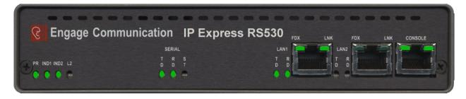
**IP-Express RS530 HS** is a Wide Area Network solution that bridges Ethernet Packets or routes the Internet Protocol through a High Speed **RS530** WAN interface that can be clocked at 16 megabits. The **RS530** WAN port supports Point to Point and Frame Relay Wide Area Networking Protocols with 24/7 proven interoperability.
