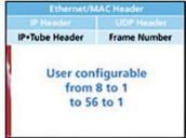
TDM over IP WAN bandwidth is not consumed by silent or redundant circuits. Note: Compression only supported with **IP•Tube GT1-C** models.
