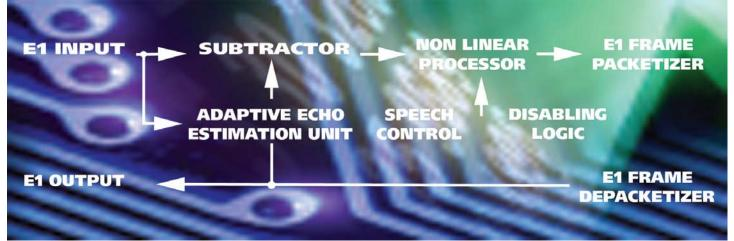
Engage's E1 Over IP products have a minimum delay configuration, 1 millisecond packetization and 4 packet buffering, which introduces a delay of 5 milliseconds. The amount of delay introduced by the packet network depends upon its switching times, packet processing, packet jitter, transmission, loading and quality of service configuration.
