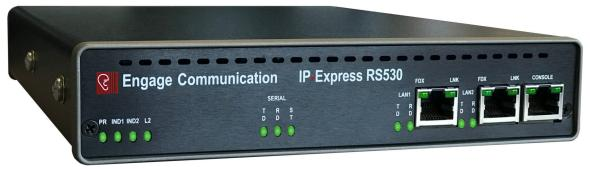
**IP-Express RS530 HS** is a Wide Area Network solution that bridges Ethernet Packets or routes the Internet Protocol through a High Speed **RS530** WAN interface that can be clocked at 16 megabits. The **RS530** WAN port supports Point to Point and Frame Relay Wide Area Networking Protocols with 24/7 proven interoperability.
