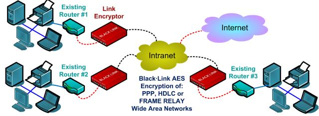
The **Black**•Link eliminates major hurdles to implementing encryption especially in contrast to the overhead, latency, and complexities of implementing a VPN encryption configuration in the WAN Router. The cost of reprogramming a WAN router can easily exceed the cost of the **Black**•Link.
